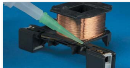
For coil termination, high temperature Rite-Lok™ Cyanoacrylate Adhesive HT700 resists continuous temperature up to 223°F (106°C) and intermittent exposure as high as 250°F (121°C).
