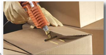
3M™ Scotch-Weld™ Hot Melt Applicator LT with 3M low temperature (265°F/129°C) adhesive effectively bonds heat-sensitive substrates such as styrene foam to itself, corrugated, or other surfaces without damaging the foam.
