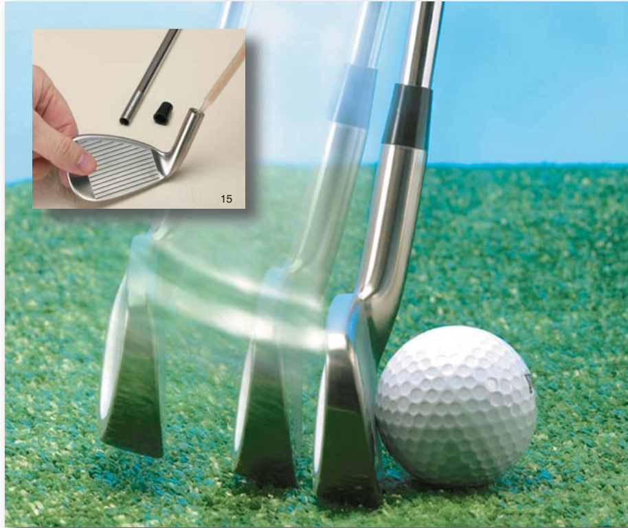
With handling strength in 2 hours and full cure in 24 hours, 3M™ Scotch-Weld™ Epoxy Adhesive DP420 bonds the shaft into the head of a golf club. Flexibility of the toughened two-part formulation helps absorb repeated impact for a secure bond. Available in 37ml, 200ml and 400ml duo-pak cartridges for use with any of the convenient hand-held 3M™ EPX™ Applicators.
