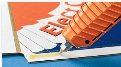
3M™ Scotch-Weld™ Hot Melt Applicator LT with 3M low temperature (265°F/129°C) adhesive effectively bonds heat-sensitive substrates such as styrene foam to itself, corrugated, or other surfaces without damaging the foam.
